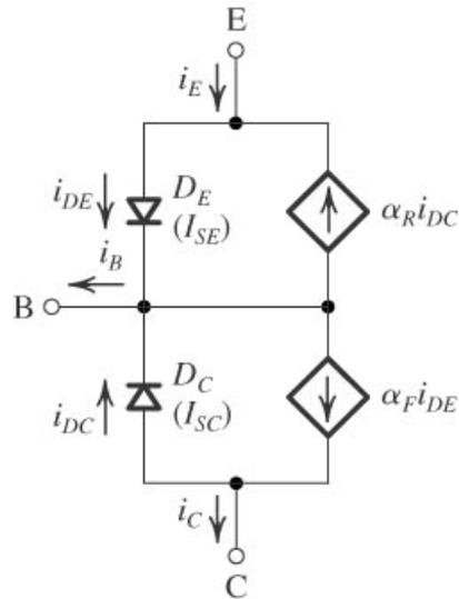
**Figure 7.15:** Ebers-Moll model of the PNP transistor.
