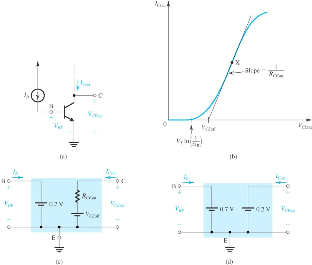
**Figure 7.21:** Equivalent circuit representation of the saturated transistor.
