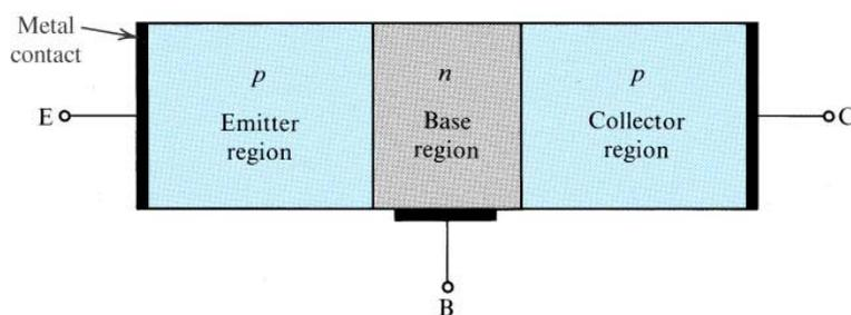
**Figure 7.5:** A simplified structure of the PNP transistor.
