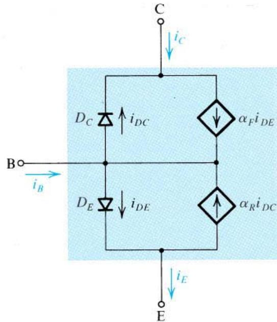
**Figure 7.11:** Ebers-Moll model of the NPN transistor.
