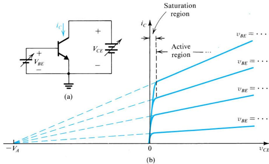
**Figure 7.17:** The  $i_C - v_{CE}$  characteristics of the BJT.
