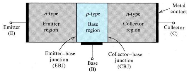
**Figure 7.2:** A simplified structure of the NPN transistor.
