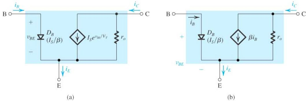
**Figure 7.18:** Large signal equivalent circuit model of an NPN BJT operating in the active mode and with common-emitter configuration.
