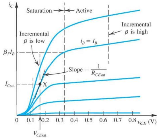
**Figure 7.19:** An expanded view of the common-emitter characteristic in the saturation region.
